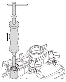
**4.** Now, a slide hammer with M16×1,5 thread can be attached.
