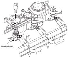
**2.** Use a 10 mm hex bit socket to remove the threaded plug.
