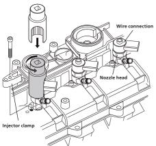
1. Remove the fuel lines and wire connections. Use a injector nozzle socket (K 430–K 434) to remove the nozzle head. Also remove the injector clamp.
