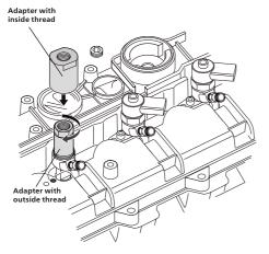
**3.** Screw the adapter with outside thread (A) onto the injector, then screw the adapter with the inside thread (B) over the first adapter.
